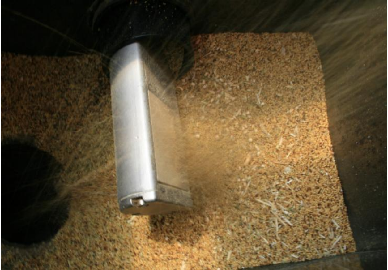
Figure 14 – Installation of the sensor in the seed stream – sensor head inside the hopper.
